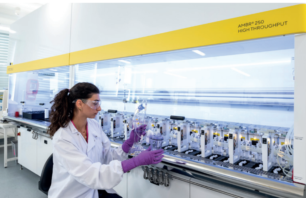
The latest-generation Sartorius Ambr® 250 HT 24 Perfusion-Enabled Bioreactor system at Celonic's Biologics Development Center (BDC) in Basel, Switzerland, supports high-throughput process development and optimization for biologics manufacturing.
