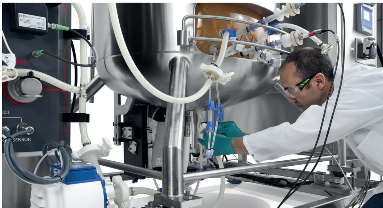
Single use 2000L bioreactor in Celonic's Heidelberg GMP facility
