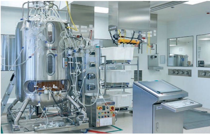
Fig. 2: The 1,000 L continuously perfused single-use production bioreactor system can be connected to an alternating tangential flow filtration cell separation device.
