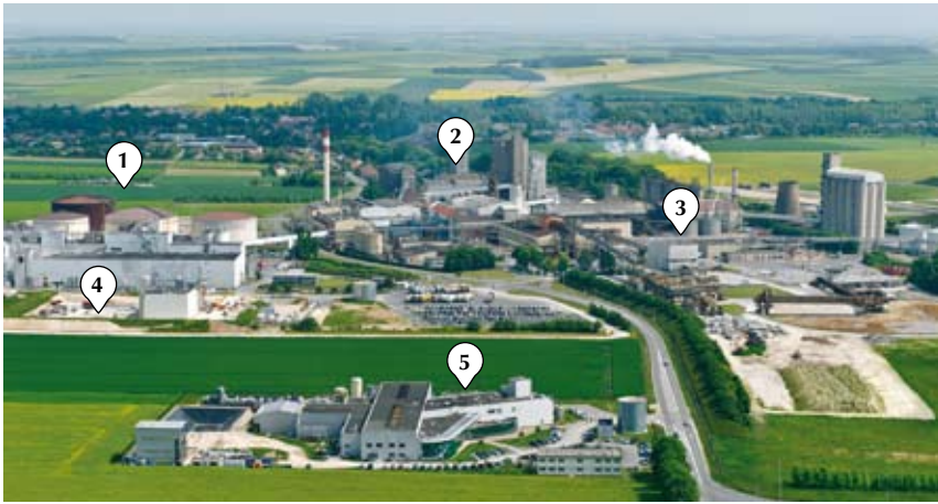
“Sohettes” biorefinery in Pomacle-Bazancourt. 1: starch/glucose production (Chamtor), 2: sugar refinement (sucrerie cooperative), 3: distillery (Christanol), 4: industrial biotech demonstration unit (A.R.D. Biodemo), succinic acid production (BioAmber), 5: Agro-industry research & development, active cosmetic ingredients (Soliance), 2 nd generation bioethanol pilot factory (Futerol), production of green surfactants (Wheatoleo), white biotech centre of excellence
